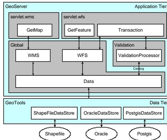
**Figure 2: GeoServer Layer Diagram with Validation Processor**
