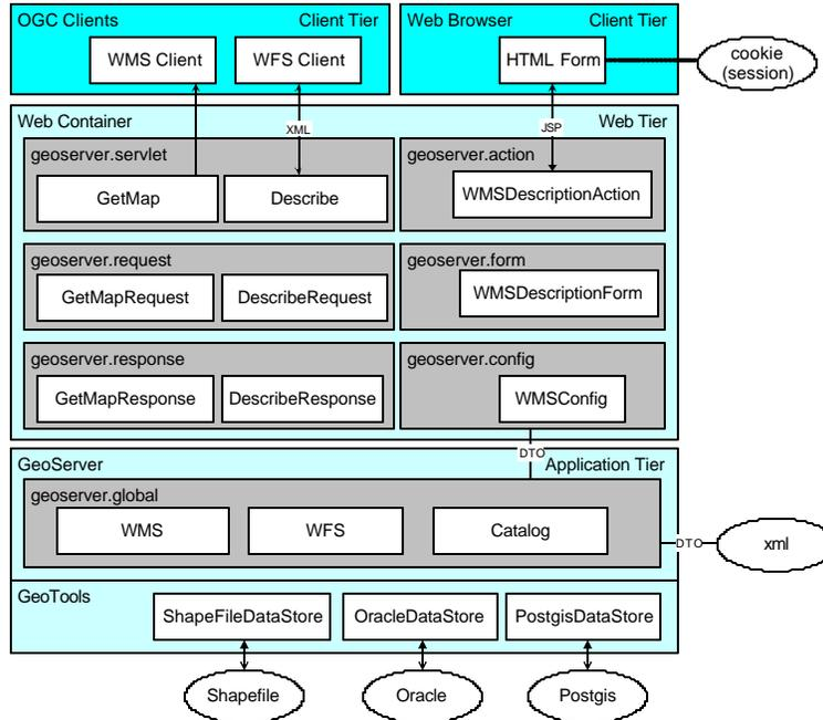
**Figure 3: GeoServer Configuration Layer Diagram**
